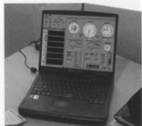
Engine and flight information is displayed and logged with RCATS software on a laptop computer in the pits. Receiver is attached to back of laptop.
