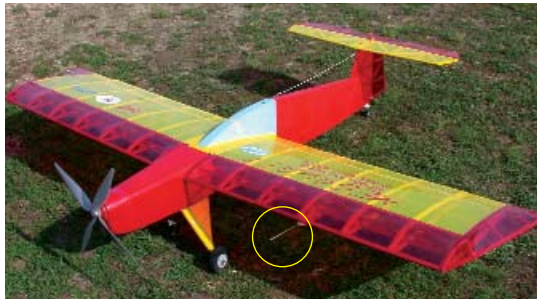
The author chose his Modelair-Tech Megawatt as the RCAT system review vehicle. The model has been flown for many years on 16-21 cells on a Power Tool (DeWalt) motor and belt drive system. The RCAT system was easily installed in this model. The 7lb. model, with 1,300 sq. in. of wing area, easily carried the 6.3 oz. system weight of the data telemetry system. With good planning, smaller models can carry the RCAT system.
