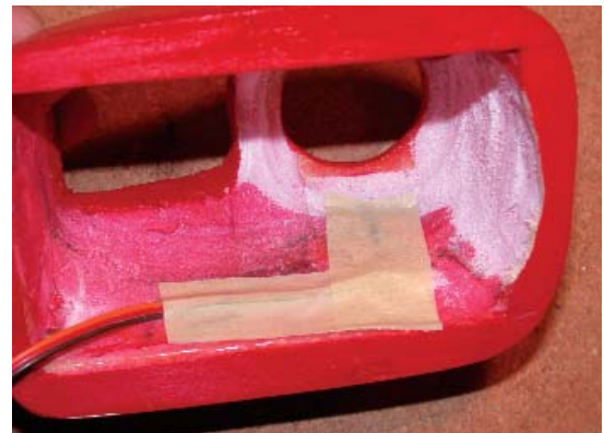
Detail of the internal wiring of the Hall sensor that measures rpm.
